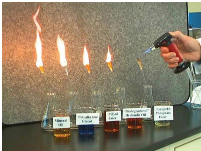
Non-phosphate ester fluids continue to burn on glass fiber wicks when ignited using a torch. Phosphate esters are not even ignited after several attempts. Photo courtesy of Eric Burkhardt.
